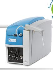
The LaserNet 200 Series allows reliability professionals to quickly and easily assess machinery health in just minutes. By testing only a few milliliters of fluid, users see a complete picture of machine wear and particulate contamination. The system offers:
