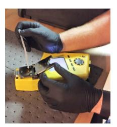
Inserting sample into Q1000 oil analyzer (NOTE: Photos are courtesy of the USCG)
