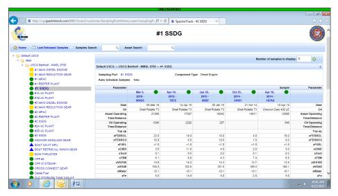
Detailed results on Ship Service Diesel Generator
