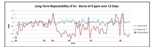
using both SpectrOil 7 and the new SpectrOil v8 software. Procedures for routine operation were followed, including restandardization when the instrument failed the daily check burns. Using the SpectrOil 7 software the instrument was restandardized 6 times in those 13 days. When the same burns were analyzed using SpectrOil v8 software, standardization was not required after the first day.
