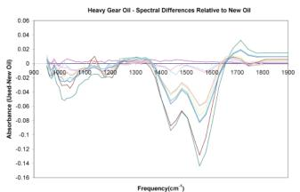
**Figure 7a:** Spectral evolution of a heavy gear oil relative to the new fluid, which shows both increasing and decreasing absorbances at various frequencies as the oil becomes more degraded.
