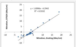
(6b): Correlation between FluidScan and ASTM D7624 for Nitration.
