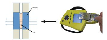
Figure 3: Fliptop cell (RHS) and schematic wedged window design (LHS).
