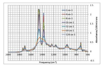
Figure 4: Overlay of oil FTIR spectra at different resolutions
