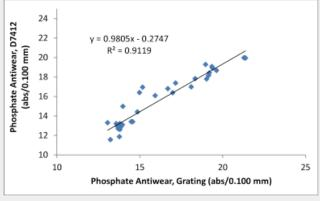
(6e): Correlation between FluidScan and ASTM D7412 for antiwear additive.
