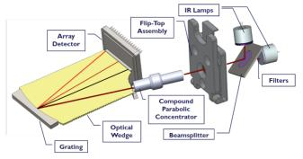
**Figure 2:** Schematic of FluidScan hardware, including IR source, fliptop cell, and grating optics. There are no moving parts in this design.
