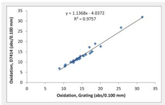
(6a): Correlation between FluidScan and ASTM D7414 for Oxidation.
