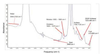
**Figure 1:** A typical infrared spectrum of in-service oil and parameters extracted from the spectrum. A laboratory FTIR spectrometer is a common tool to provide such information. A lab technician or data analyst then interprets the spectrum and provides quantitative information about the oil condition.
