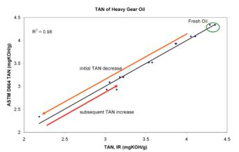
**Figure 7b:** Relationship between ASTM D664 and infrared TAN values for a heavy gear oil. This oil has a complicated evolution where the fresh oil's TAN initially decreases down to a minimum level, then begins to increase towards a maximum alarm value.
