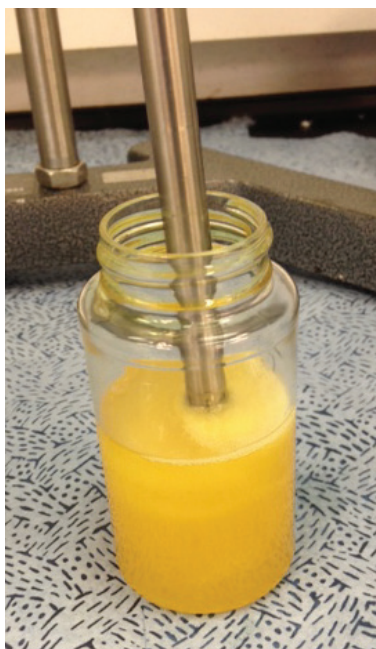
Figure 4. Homogenizing a sample of water-contaminated oil.
