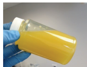
Figure 7. Sample which was shaken vigorously by hand for 30 seconds. To the eye, the opacity looks similar to the homogenized samples even though the water is not uniformly dispersed in the sample.
