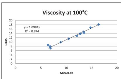
Figure 10. Comparison of Viscosity measurements between MicroLab and Lab D445 for a series of fresh Shell Omala oils with grade from ISO46 to ISO 320..
