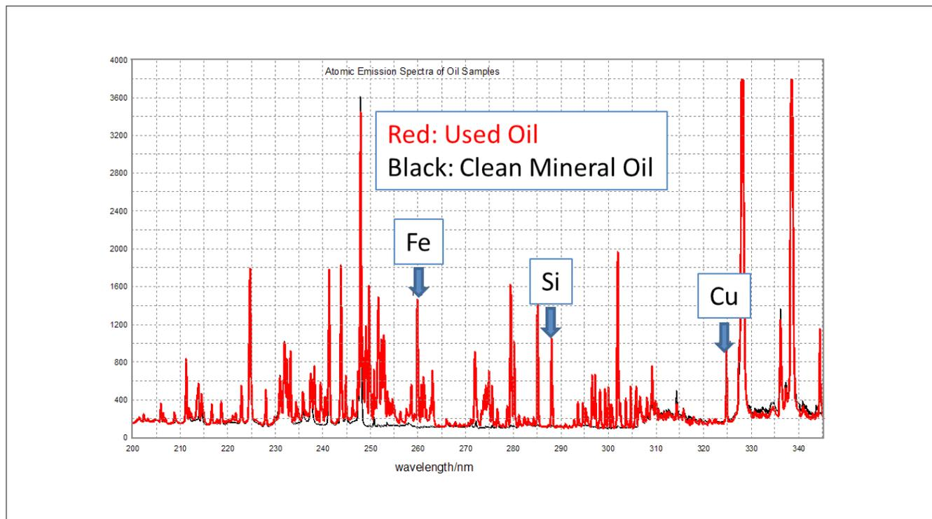
Figure 3. Representative emission spectra from two oil samples: the spectrum in red is from a customer used oil sample and the one in black is white mineral oil shown here for comparison.
