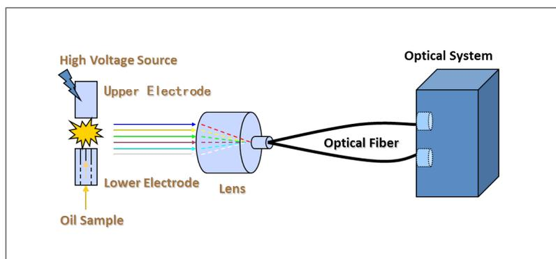
Figure 2. Schematic of MicroLab OES system and a picture of spark stand (above).
