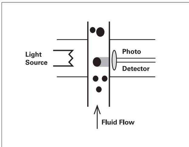
Figure 12. The light blocking particle counter module in the MicroLab.
