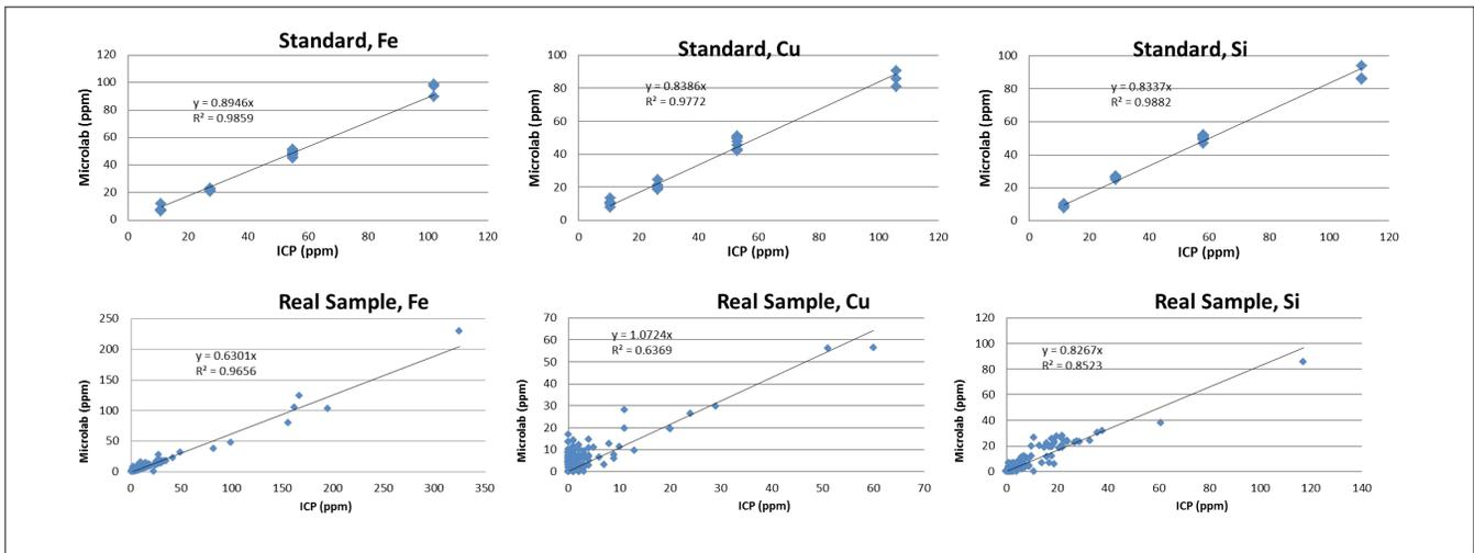
Figure 4. MicroLab results compared to Lab ICP-OES for elemental standards and several real in-service oil samples.
