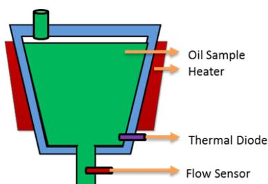
Figure 9. The dual viscosity module in the MicroLab.
