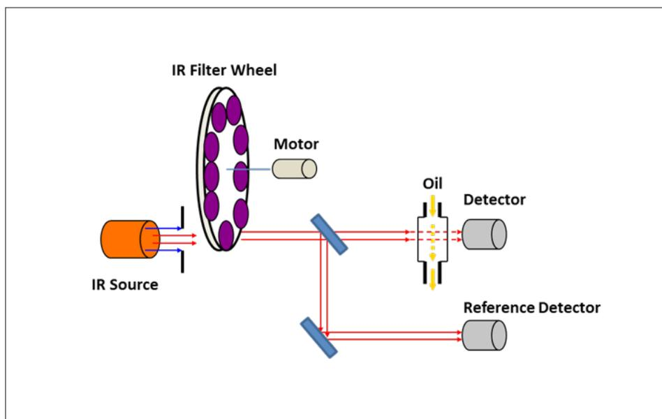
Figure 6. The IR module inside the MicroLab.
