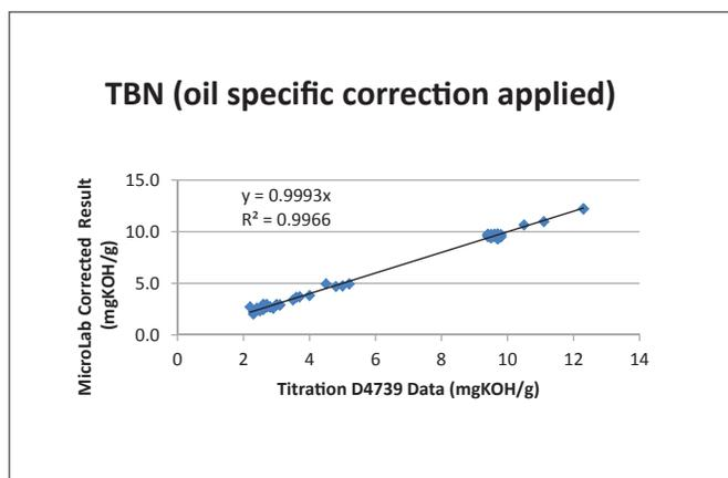
Figure 8. Applying an oil-specific slope and offset to TBN results improves the accuracy and correlation to the laboratory D4739 method.
