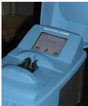
Oil viscosity results are visible in the Q3000 display.
