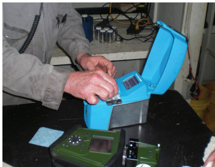
Testing air compressor oil aboard the USNS Watson, using the Q3000
