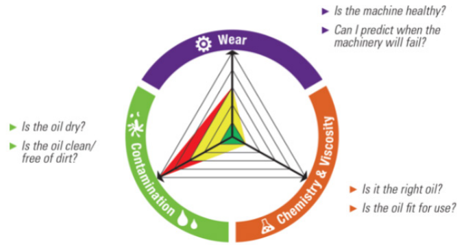
Figure 2: Trivector™ oil analysis: A powerful way to summarize data from all 3 facets of oil analysis by graphically illustrating direction and severity of faults, enabling quick decision making
