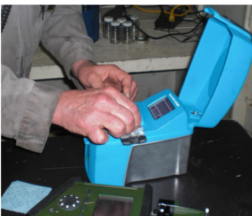
Figure 2: Fluidscan and Minivisc combo kit is widely used for onboard monitoring today
