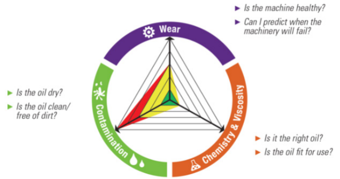
Figure 3: Trivector™ oil analysis: A powerful way to summarize data from all 3 facets of oil analysis by graphically illustrating direction and severity of faults, enabling quick decision making
