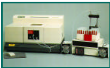
FT-IR Spectrometer Lubricant Physical Property Analysis
